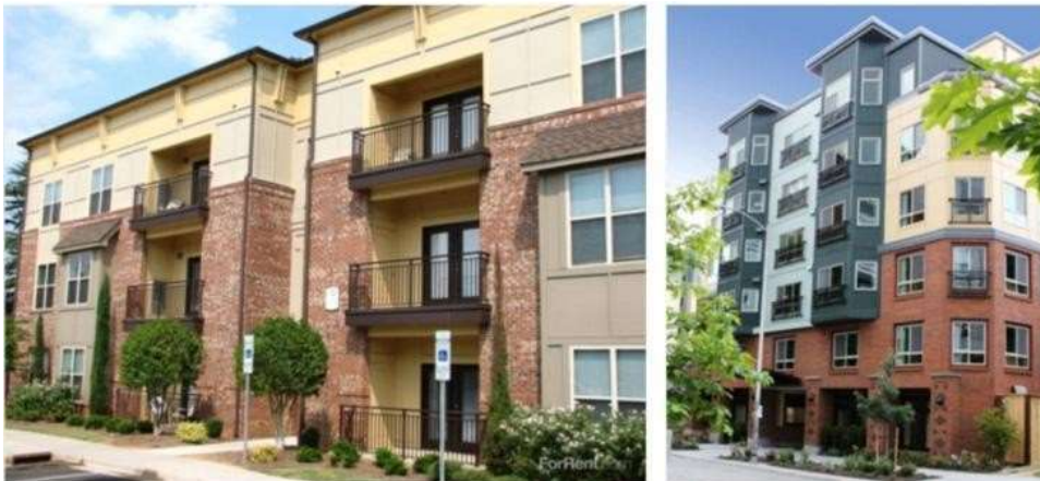
Figure E.3.1.e. Examples of articulation of multifamily residential building facades. All examples use window fenestration and vertical building modulation elements. The upper examples use a mixture of material changes and detail components to further articulate the facades. In the lower left example, the balcony element's dramatic mix of color, material, and projection are effective in meeting the standards. The lower right example adds a combination of materials, color changes, and building modulation to help meet the following standards.
