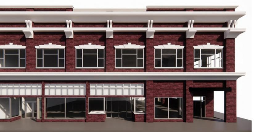
WITH THE INSTALLATION OF BRICK VENEER TO MATCHING THE EXISTING BUILDING, UPPER FACADE WINDOWS, A FRESH COAT OF PAINT, NEW AWNINGS AND A RECONFIGURE OF THE CORNER ENTRANCE, THE FULLER-QUIGG BUILDING WILL CONTINUE TO BE ONE OF THE MOST ICONIC BUILDINGS IN DOWNTOWN WENATCHEE.
