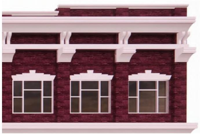
THE BUILDINGS ORIGINAL WINDOW ANCON BRACKETS HAVE BECOME WEATHERED OVER TIME, RESULTING IN A LESS VISIBLE ATTRIBUTE OF DESIGN. FOR THE FACADE UPDATES IT IS BEING PROPOSED THAT THE ORIGINAL WINDOW PEDIMENTS AND SILLS REMAIN, BUT THE ANCON BRACKETS RECEIVE A FRESH COAT OF PAINT TO MATCH THE OTHER DESIGN ELEMENTS OF THE BUILDING.
