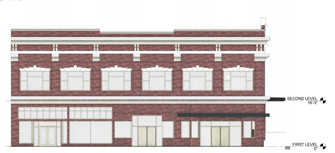
2 SOUTH ELEVATION- NEW SCALE: 1/8" = 1'-O"
