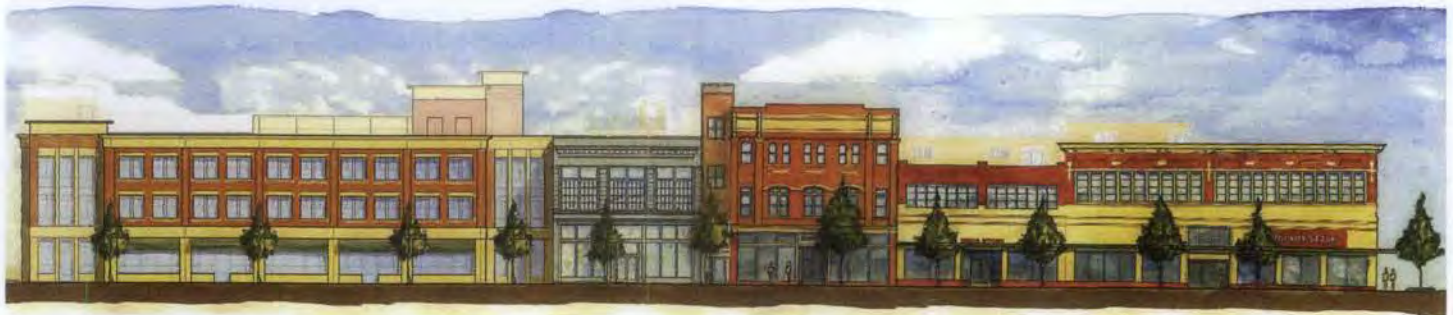
Figure 22. The proposed new addition is compatible with the historic buildings that remain on the block. Its design with multiple storefronts helps break up the mass.
