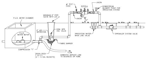
All connections to the domestic service water line must be at least 3 feet away from the meter chamber. Most domestic water lines are located 3 to 4 feet below ground. You must contact the correct water purveyor to arrange for the water to be shut off inside the water meter chamber. Entering the water chamber or shutting the water service off within the meter chamber is <u>prohibited</u>.
