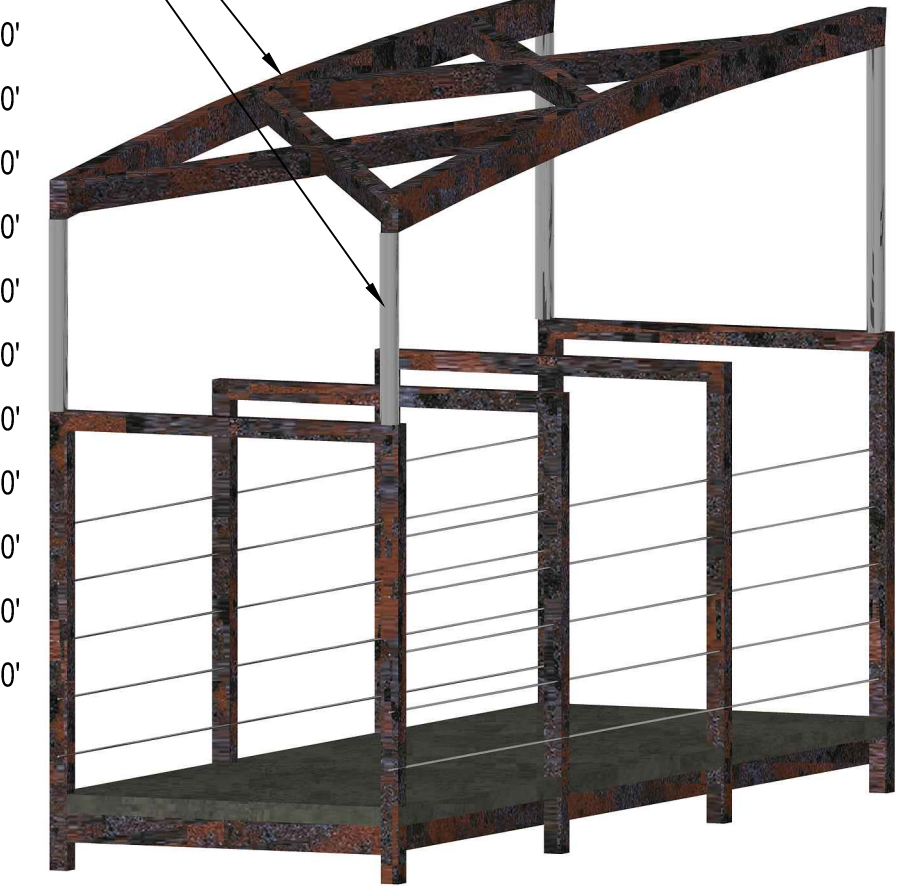
TUNABLE TRUSS SECTION
