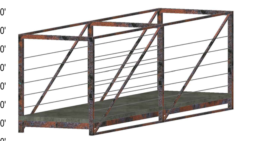
HIGH STRENGTH WEATHERING STEEL TRUSS SECTION
