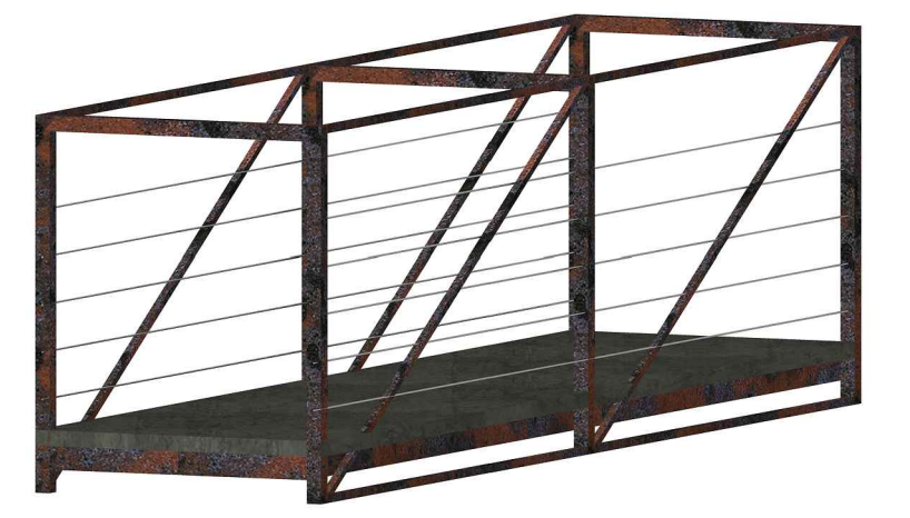
WEATHERING STEEL TRUSS SECTION
