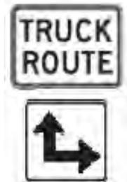
The intersection sign should be placed at the intersection of freight routes as well as in advance of the intersection in order to give drivers adequate time for deceleration or lane changes. Advanced signing should be placed a minimum of 150 feet from intersections on arterial and collector roadways with a posted speed of 35 mph or below, and 350 feet for arterial and collector roadways with posted speeds of 40 mph or greater.
