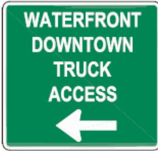
Trailblazer or guide signing should be used to direct trucks to freight routes or to provide advanced notice of prohibitions or complex situations. An example would be alerting trucks of the need to use a certain lane in preparation for a required turning movement. Trailblazer/Guide signs should consist of white lettering on a green background.
