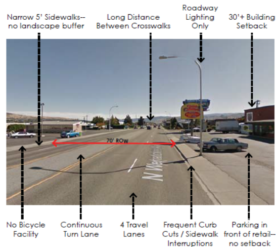
Existing Street Cross Section
