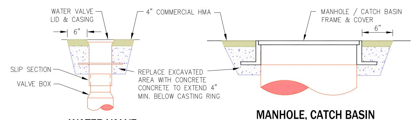
WATER VALVE **ADJUSTMENT DETAIL**
