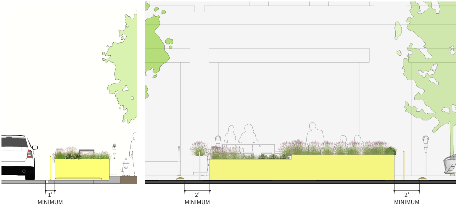
Required end and street-side buffers
