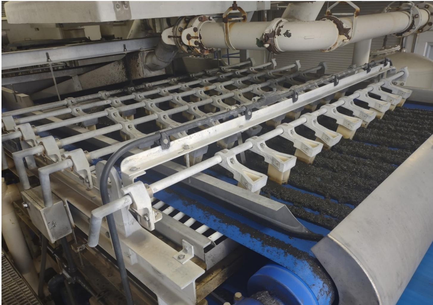
Next, the biosolids are compressed between the two belts which are then fed through a series of rollers. The excess water drains out the bottom of the equipment.
