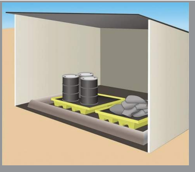
Store hazardous materials/wastes inside secondary containment structures under cover and protected from rainfall. (Source: Idaho Construction Site Erosion and Sediment Control Field Guide)
