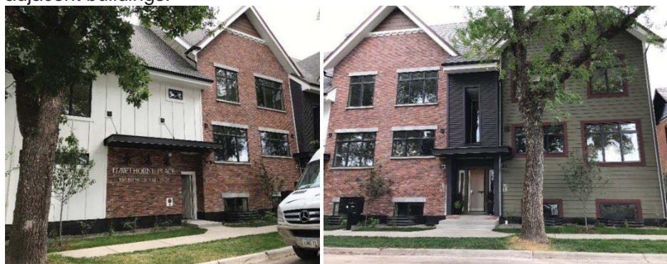
The above building uses fiber cementitious wall-board panels and planks in different textures and colors to help articulate the façade. The white color replicates the board and batten style in the left image and green color in the right image effectively replicates horizontal wood siding.
