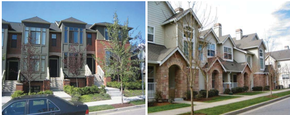
Figure E.3.1.c. The units in the left image each have distinct, but identical windows and roof forms. The outside unit on the right is differentiated through the use of building materials, window design, unit size, and façade detailing. The units in the right example include reverse elevations that add to the building's composition.
