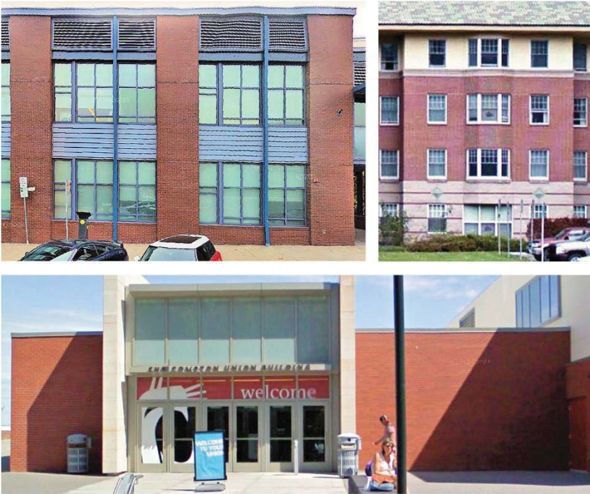
Figure 10.36.050(4)(ed)(vi). Portions of front building facades illustrating the percentages of transparent fenestration (clear, transparent windows and doors). The upper left and lower examples feature about 35% transparency. The one on the upper right features about 25% transparency
