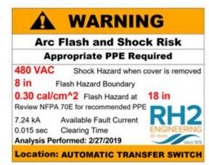
device coordination and arc flash calculations for equipment at each location. This report will make recommendations to equipment settings along with recommendations for equipment replacements where needed. Lastly, RH2 will produce arc flash hazard warning labeling, for installation by the City, to meet the requirements of National Fire Protection Association (NFPA) 70E and the Washington Administrative Code.
