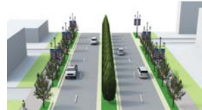
A: Four Lane Roadway with Continuous Landscaped Median
