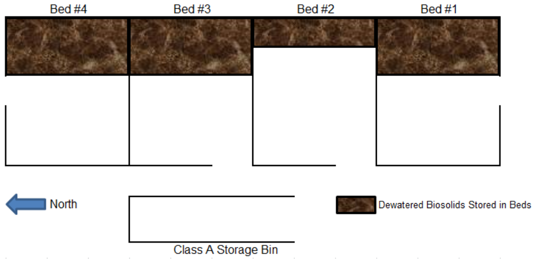
Figure 4-3. Dewatered Solids Stored in Drying Beds at the End of Non-Drying Season
