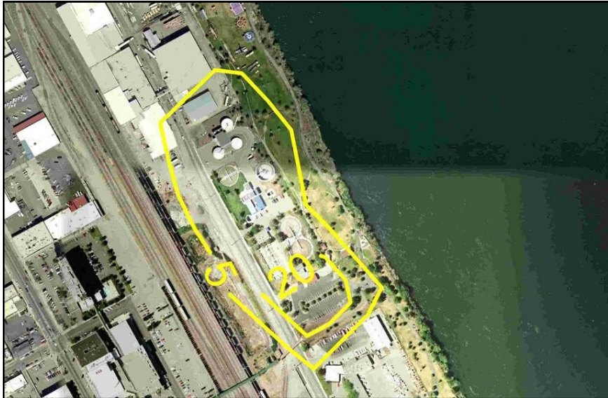
Drawing showing target odor isopleths...or “iso-stink” lines
