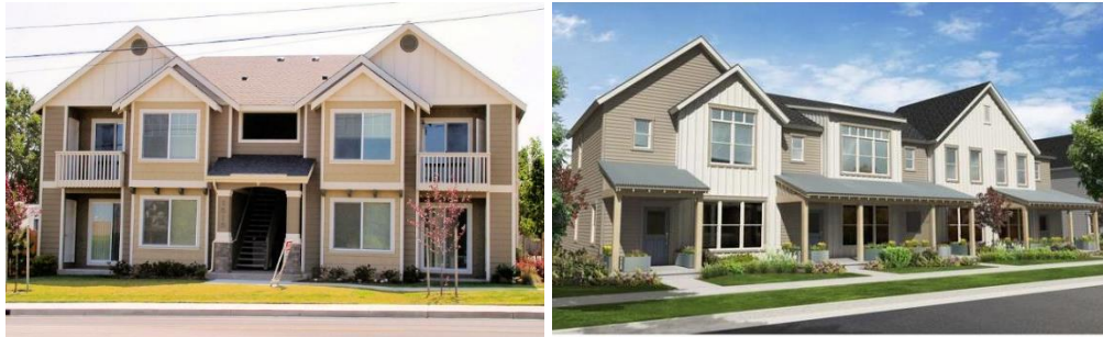
Figure E.3.1.b. Two examples of modulation effectively used on a duplex (left) and a triplex (right).
