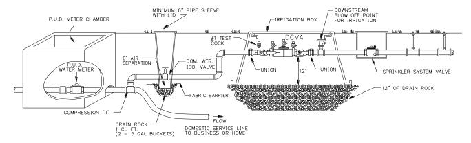
All connections to the domestic service water line must be at least 3 feet away from the meter chamber. Most domestic water lines are located 3 to 4 feet below ground. You must contact the correct water purveyor to arrange for the water to be shut off inside the water meter chamber. Entering the water chamber or shutting the water service off within the meter chamber is <u>prohibited</u>.
